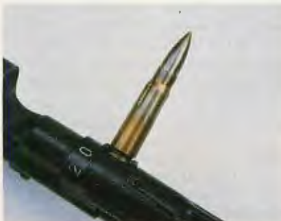
Type 81 series gas regulator is easily adjusted with the base of a cartridge, even while hot.
